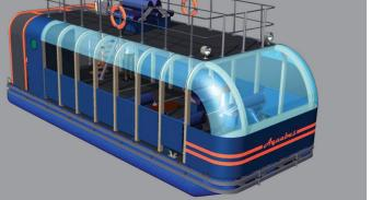
It is a mini ferry which can carry 12-24 persons. May be equipped with a fixed roof and "sides", protecting passengers from wind and rain.
