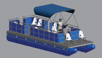
Main technical data: Length – from 6 to 12 m Width – from 2,5 to 4 m Height – up to 2,9 m Freeboard deck – 0,5 m
